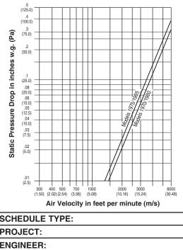
Tested per AMCA Standard 500-D using test set-up Figure 5.3, ductwork upstream and downstream.
