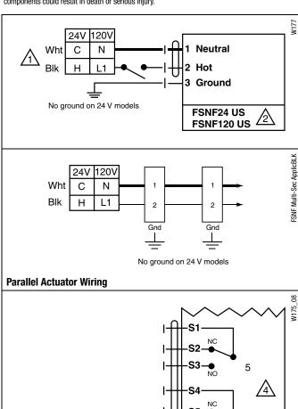
Auxiliary switch wiring for FSNF24-S US, FSNF120-S US
