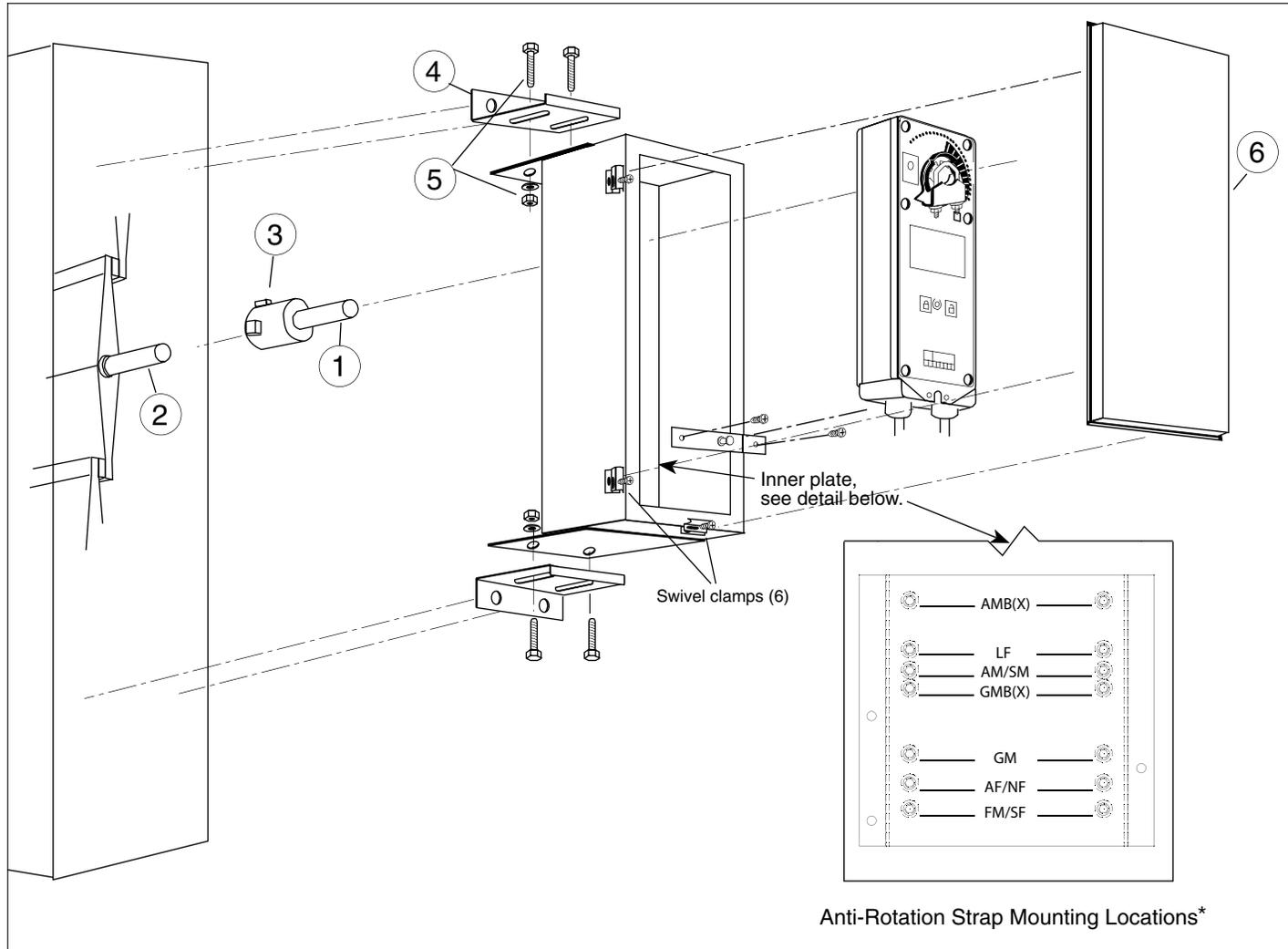
\*AFB, AFX, NFB and NFX can be installed using GM mounting location without the need of the Z-AF retrofit bracket.
